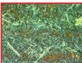
Color etching – martensitic structure (500x magnification)
