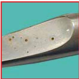
Chloride-induced pitting on instrument.
