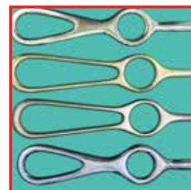
Titanium oxide discoloration occurs mostly on reflective surfaces over large surfaces, yellow-brown to blue-violet, sometimes with a shimmering appearance, in the wash chamber or over the entire surface of the instrument during machine-cleaning.
