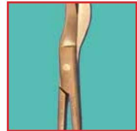
Etching effect on surface of instrument. Cause: Effects of over-dosed acids.
