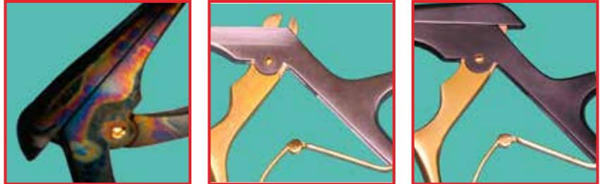
Example: black, TiAlN coated punch. The partial erosion of the layer has caused bright, colorful discoloration or complete removal of the layer with undamaged gold-plated components.
