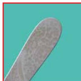
Typical silicate discoloration occurs, regardless of the nature of the surface, over large surfaces, yellow-brown to blue-violet in the cleaning & disinfection process, or in spots, droplet-shaped with pronounced condensation stain-like appearance during the steam sterilization process.
