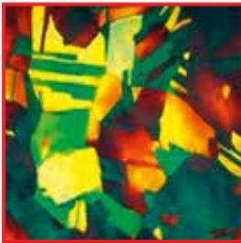
Color etching - austenitic microstructure on rust and acid-resistant instrument steel (500x magnification)
