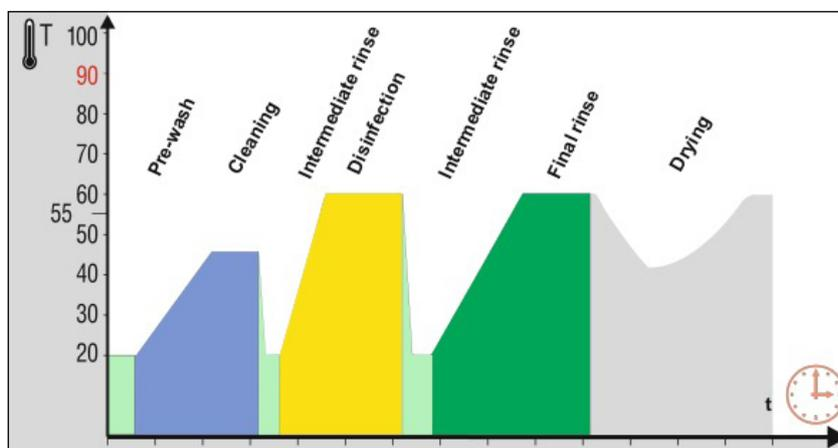
Cleaning program with chemo-thermal disinfection for heat-sensitive endoscopes
