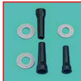
Right: Swollen seals caused by incorrectly applied instrument oil.
